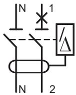
**en** Residual Current Circuit Breaker with Overcurrent Protection (RCBO) provides:
