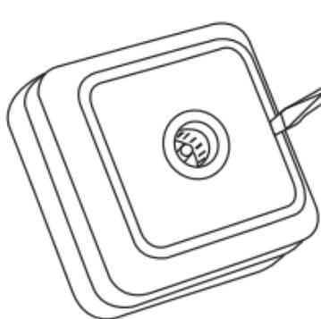
Remove the front panel by pushing the flat screwdriver tip into the side grooves between the cover and the front panel of the housing.
